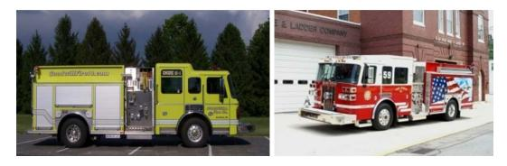
**E54-4 and E56-1** serves primarily as a rural water supply units. They are frequently requested as supply units in Maryland. E54-4 carries several hundred feet of large diameter hose (LDH) and both engines are used in areas that lack hydrants.
